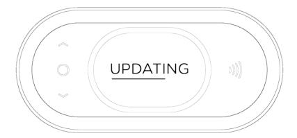
If successful, the PillDrill Hub will either show an updating screen or move directly into your account showing the clock screen. It is normal for the light ring to blink several colors and if you have a slow internet connection, this process can take up to 5 minutes.
